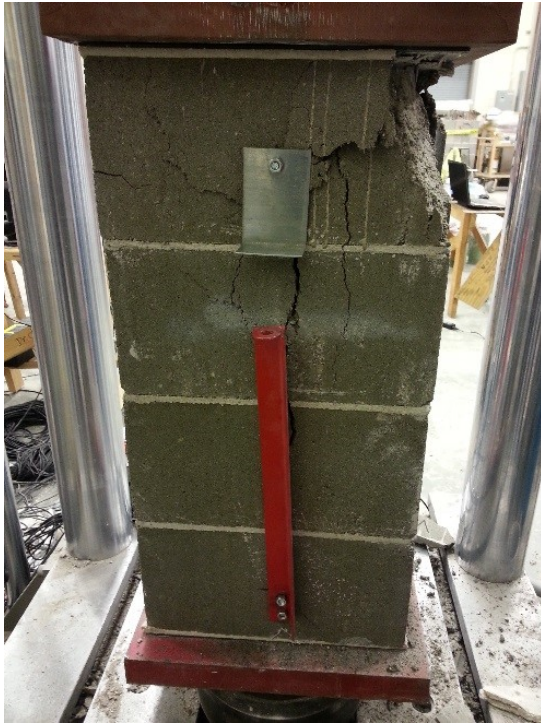
(a) Backside of 37% Rubber CMU
